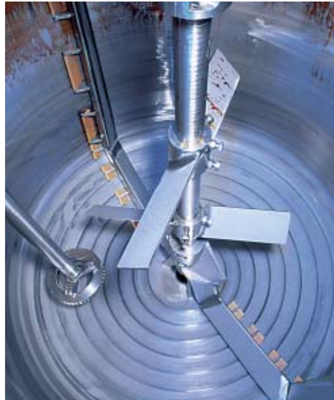
Quality on every scale. The formulations are mixed in large blending tanks by agitators, then finally filled off.
