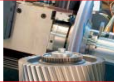
Gear grinding with MEBA cutting oil.
