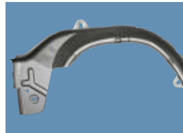
Deep drawing of wheel arches with Platinol B 804/3 COW.
